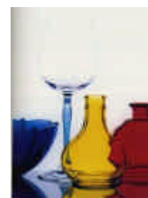
Figure 4. Glass ware demonstrating the still glassy appearance of crystal glass and other types of glasses after being spray coated with hybrid, sol-gel derived layers
